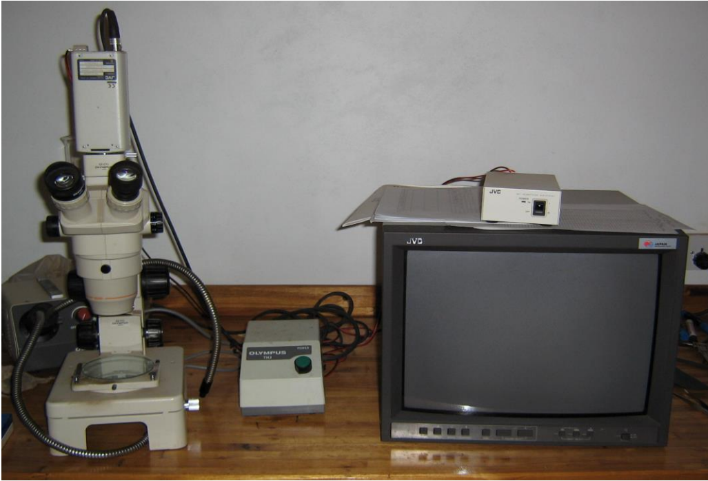
Figure 3.2. A compound microscope connected to a video display system used for viewing the Lethrinops gosseii transverse sectioned sagitta otoliths.
