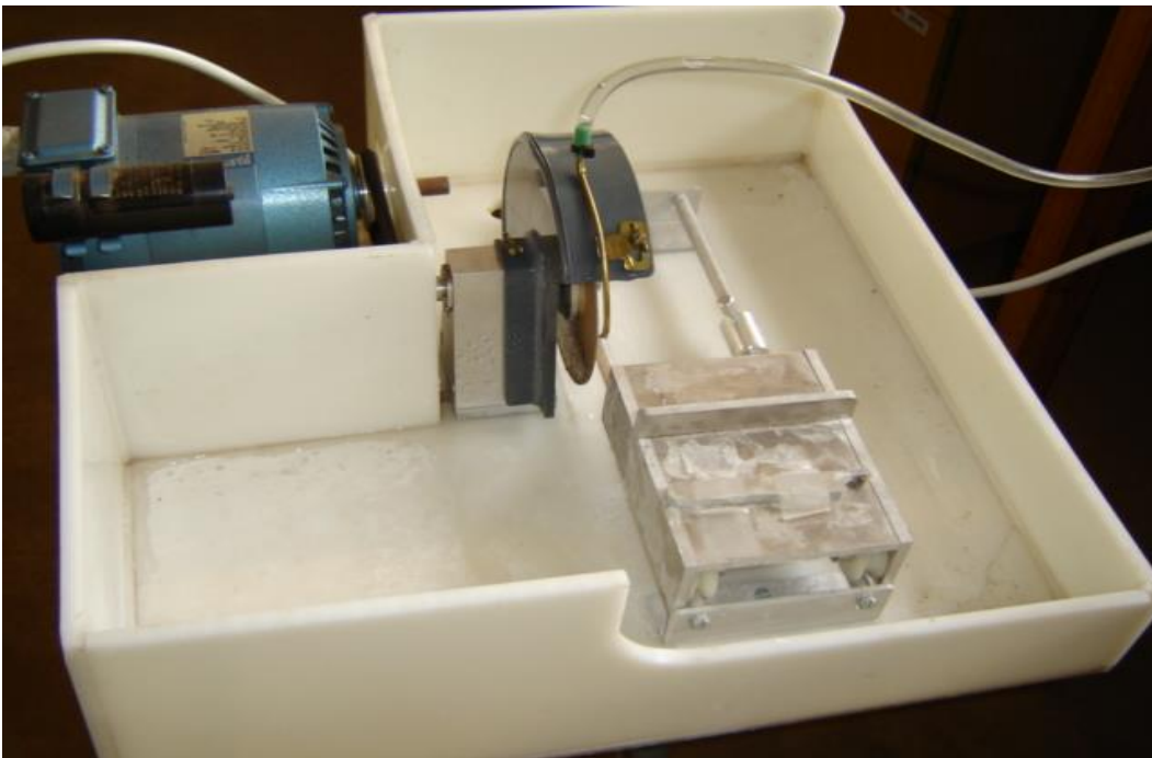
Figure 3.1. An otolith cutter with a dual blade high-speed diamond saw used for cutting thin transverse sections of Lethrinops gossei sagitta otoliths.
